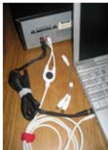
*These cables have stereo jack at one end and RCA jacks at the other. The small cable converts the RCA down to the stereo jack. The white cable is OUT from computer to IN of recorder. The black in OUT from recorder to IN of computer.*
