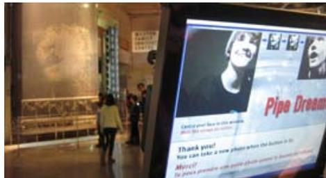
at the right, takes your photo, displays it on the screen (small photo right side) and then recreates a larger version image in bubbles in hundreds of vertical tubes (left and in rear). The bubbles continue to rise and the photo disappears. You have to be careful to capture the image in low and varied lighting conditions.
